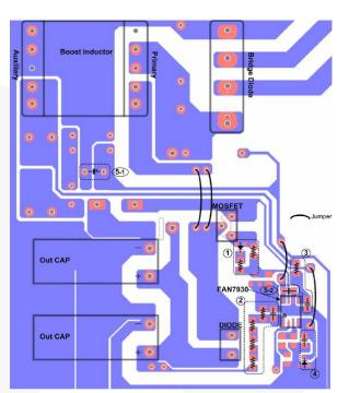
Figure 44. Recommended PCB Layout
