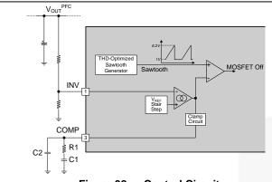
Figure 32. Control Circuit
