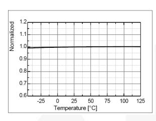
Figure 4. Voltage Feedback Input Threshold 1 (V<sub>REF1</sub>) vs. T<sub>A</sub>
