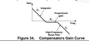
For the transconductance error amplifier side, gain changes based on differential input. When the error is large, gain is large to suppress the output dip or peak quickly. When the error is small, low gain is used to improve power factor performance.
