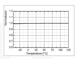
Figure 5. Start Threshold Voltage (VSTART) vs. TA
