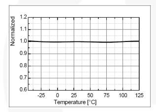
Figure 12. Maximum On-Time Program 2 (t<sub>ON,MAX2</sub>) vs. T<sub>A</sub>
