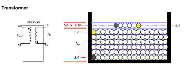
Figure 46. Transformer Schematic Diagram
