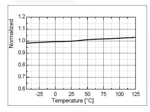
Figure 14. Input High Clamp Voltage (V<sub>CLAMPH</sub>) vs. T<sub>A</sub>
