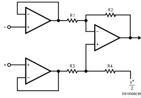
FIGURE 8. Three-op-amp Instrumentation Amplifier
