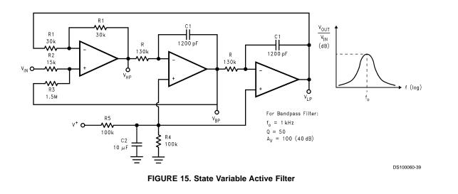
$$V_{LP} = \left(\frac{2R_{3}}{R_{2} + R_{3}}\right) \frac{\frac{1}{R^{2}C^{2}}}{S^{2} + \frac{1}{\left(\frac{R_{2} + R_{3}}{2R_{2}}\right)RC}S + \frac{1}{R^{2}C^{2}}} V_{IN}$$
