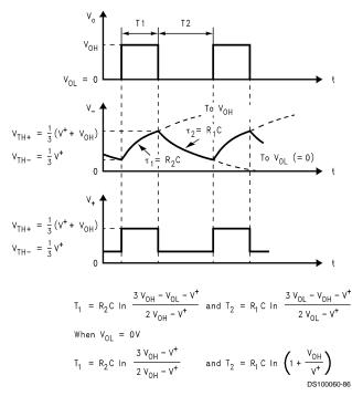
FIGURE 17. Waveforms of the Circuit in Figure 16
