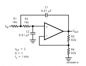
FIGURE 13. Sallen-Key 2nd-Order Active Low-Pass Filter
