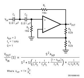
FIGURE 14. Sallen-Key 2nd-Order Active High-Pass Filter
