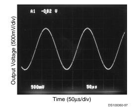
FIGURE 1. Output Swing of LMV324
