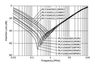
Common Mode Insertion Loss (Typ.)
