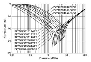
Differential Mode Insertion Loss (Typ.)
