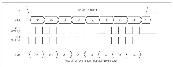
Figure 16. SPI Clocking Modes
