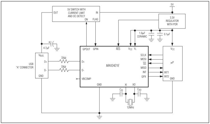
Figure 21. MAX3421E in a Host Application
