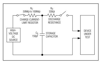
Figure 24. IEC 61000-4-2 ESD Test Model
