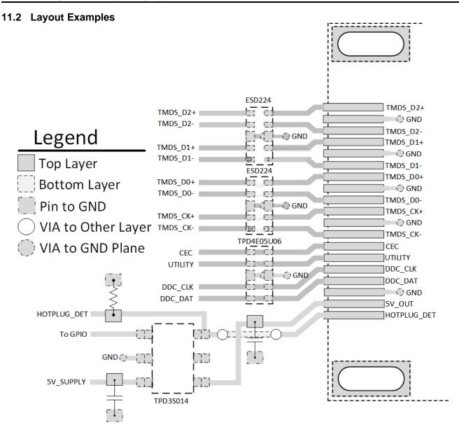
Figure 15. HDMI Type-A Transmitter Port Layout
