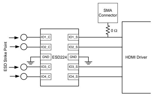
Figure 11. System Level IEC 61000-4-2 ESD Test Setup with ESD224 protecting an HDMI driver chip
