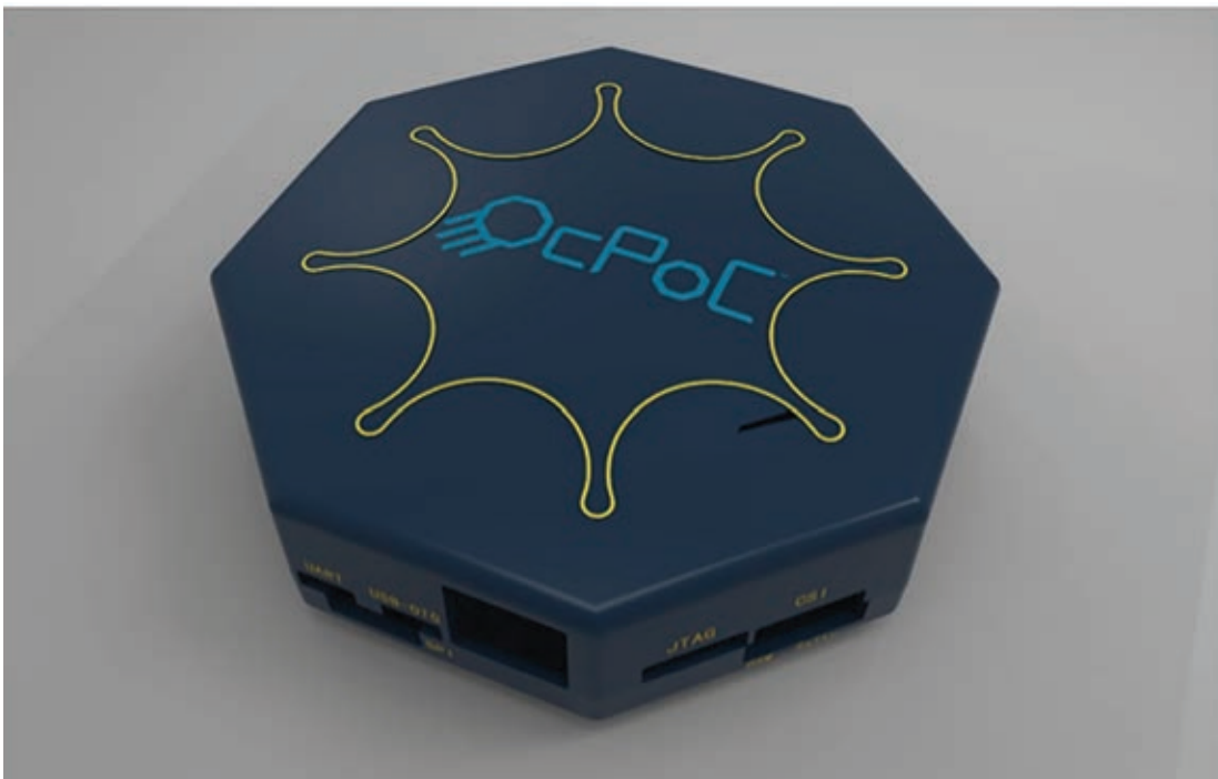
Figure 2 – The OcPoC system will be the first commercially available flight control platform powered by the Zynq SoC chip.
