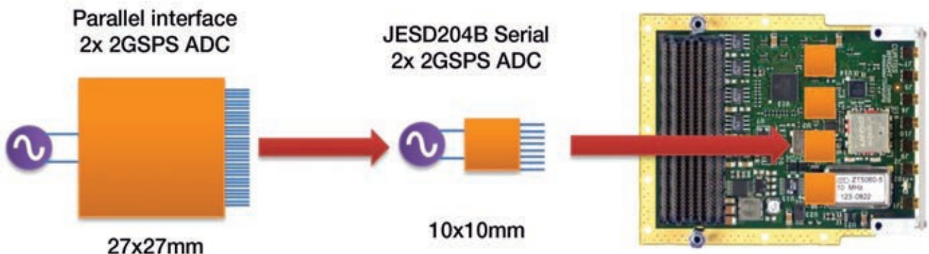
Figure 1 – The effect of package shrink on FMC through JESD204B
