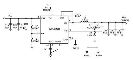
Figure 9:  $V_{IN} = 19V$ ,  $V_{OUT} = 5V/6.5A$
