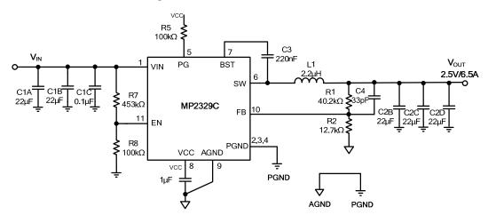
Figure 11:  $V_{IN} = 19V$ ,  $V_{OUT} = 2.5V/6.5A$
