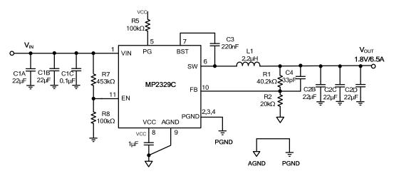
Figure 12:  $V_{IN} = 19V$ ,  $V_{OUT} = 1.8V/6.5A$
