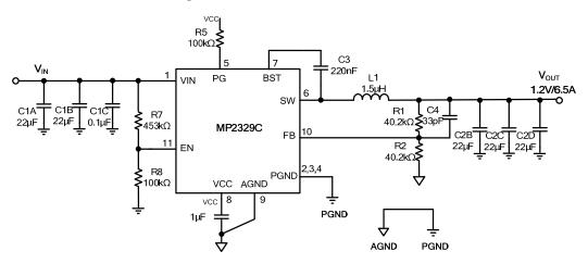
Figure 14:  $V_{IN} = 19V$ ,  $V_{OUT} = 1.2V/6.5A$
