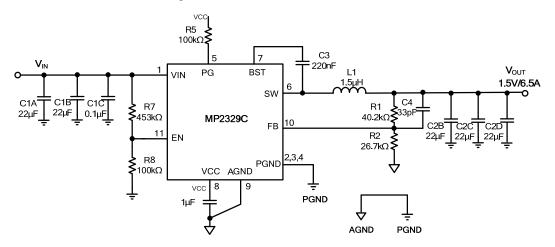
Figure 13:  $V_{IN} = 19V$ ,  $V_{OUT} = 1.5V/6.5A$
