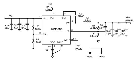
Figure 15: V<sub>IN</sub> = 19V, V<sub>OUT</sub> = 1V/6.5A
