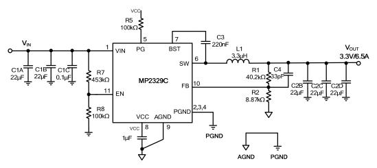
Figure 10:  $V_{IN} = 19V$ ,  $V_{OUT} = 3.3V/6.5A$
