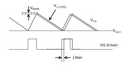
Figure 2: Jitter in PWM Mode
