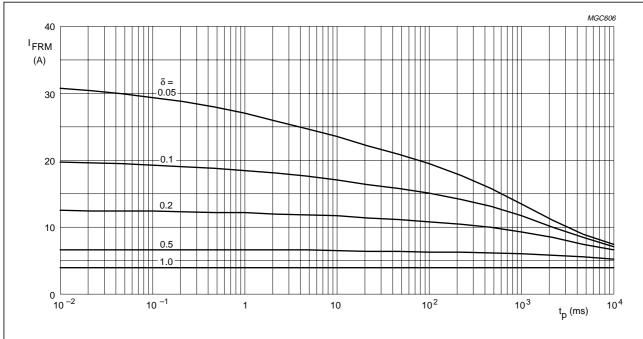
$T_{tp}$  = 60 °C;  $R_{th j-tp}$  = 25 K/W.
