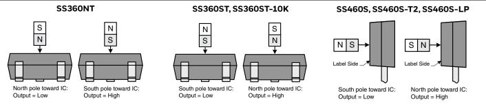
SS360NT, SS360ST, SS360ST-10K, SS460S, SS460S-T2, SS460S-LP
