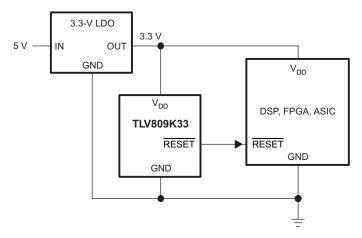
Figure 10. Monitoring a 3.3-V Supply
