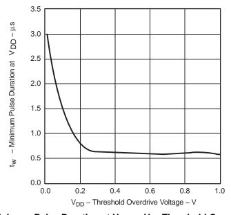
Figure 11. Minimum Pulse Duration at V<sub>DD</sub> vs V<sub>DD</sub> Threshold Overdrive Voltage
