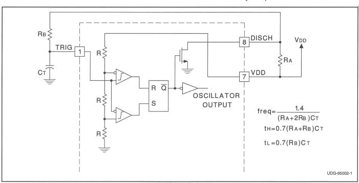
Figure 1. Oscillator Block Diagram
