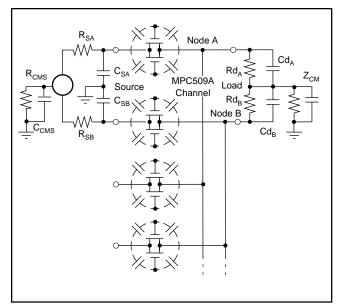
FIGURE 4. Settling and Common-Mode-Effects—MPC509A
