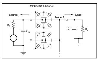
FIGURE 3. Settling Time Effects—MPC508A
