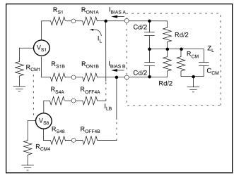
FIGURE 2. MPC509A DC Accuracy Equivalent Circuit.
