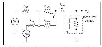
FIGURE 1. MPC508A DC Accuracy Equivalent Circuit.
