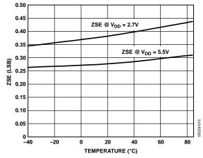
Figure 14. Zero-Scale Error vs. Temperature
