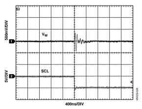
Figure 27. Digital Feedthrough
