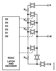
Figure 37. AD5258 Equivalent RDAC Circuit
