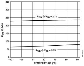
Figure 19. R<sub>WB</sub> vs. Temperature
