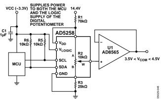
Figure 44. Circuitry When a Separate Supply Is Not Available for VDD
