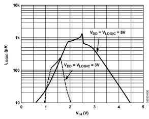
Figure 25. Logic Supply Current vs. Input Voltage
