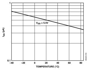
Figure 15. Supply Current vs. Temperature
