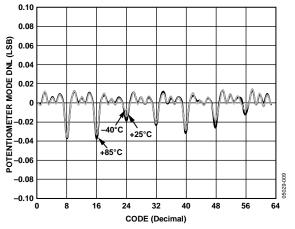
Figure 8. DNL vs. Code vs. Temperature
