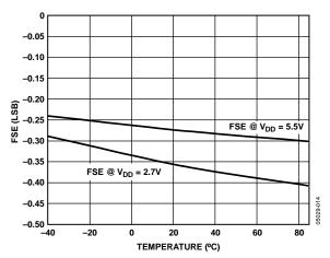
Figure 13. Full-Scale Error vs. Temperature
