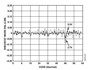
Figure 6. R-DNL vs. Code vs. Supply Voltages
