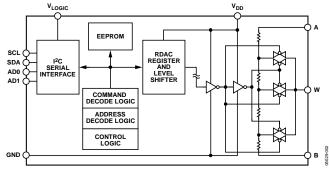
Figure 2. Block Diagram Showing Level Shifters
