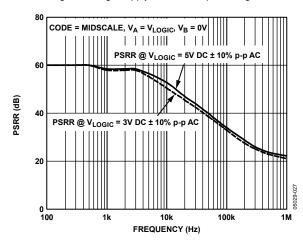
Figure 26. Power Supply Rejection Ratio vs. Frequency
