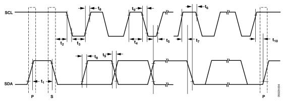
Figure 3. I<sup>2</sup>C Interface Timing Diagram
