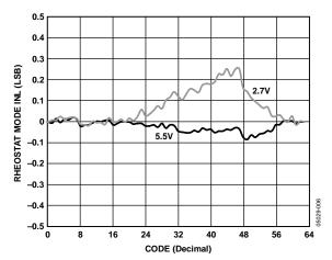
Figure 5. R-INL vs. Code vs. Supply Voltages
