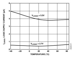
Figure 16. Logic Supply Current vs. Temperature vs. VLOGIC
