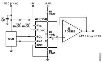
Figure 43. V<sub>COM</sub> Adjustment Application
