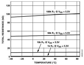
Figure 20. Total Resistance vs. Temperature
