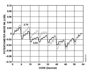
Figure 9. INL vs. Code vs. Supply Voltages
