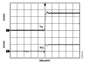
Figure 29. Large-Signal Settling Time
