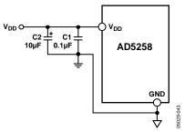
Figure 42. Power Supply Bypassing
