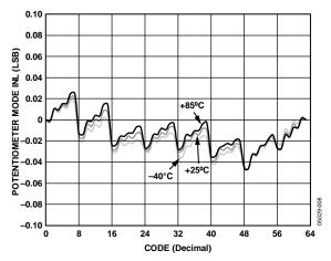
Figure 7. INL vs. Code vs. Temperature
