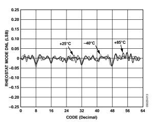
Figure 12. R-DNL vs. Code vs. Temperature
