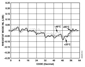
Figure 11. R-INL vs. Code vs. Temperature
