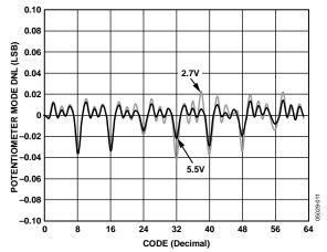
Figure 10. DNL vs. Code vs. Supply Voltages
