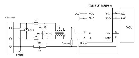
Fig. 2: Port protection circuit for harsh environments
