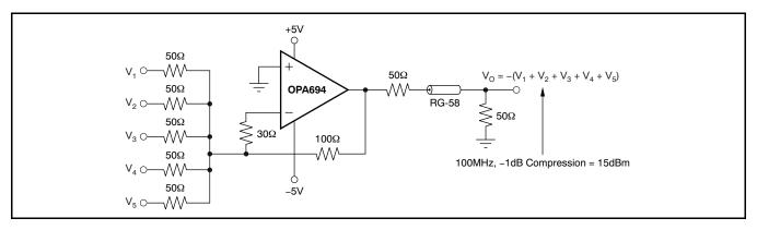
Figure 34. 200MHz RF Summing Amplifier
