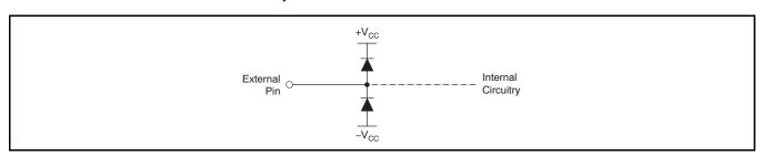
Figure 42. Internal ESD Protection
