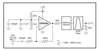
Figure 35. IF Amplifier Driving SAW Filter
