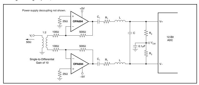
Figure 33. Wideband, AC-Coupled, Low-Power ADC Driver
