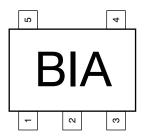
Pin Orientation/Package Marking
