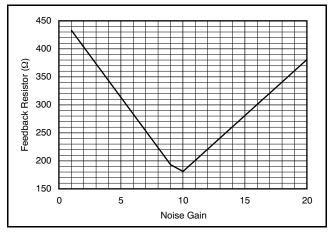
Figure 39. Feedback Resistor vs Noise Gain
