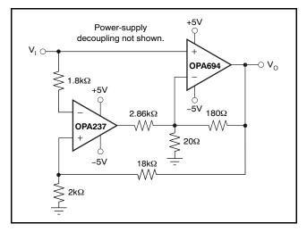
Figure 41. Wideband, DC-Connected Composite Circuit
