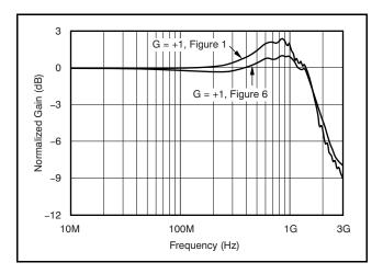
Figure 37. Gain of +1 Frequency Response
