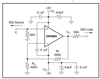
Figure 31. DC-Coupled, G = +2, Bipolar-Supply Specification and Test Circuit
