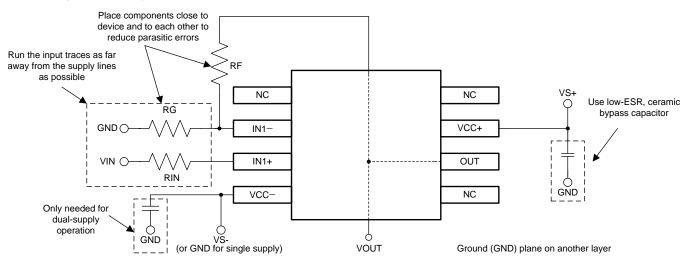
Figure 7. Operational Amplifier Board Layout for Noninverting Configuration
