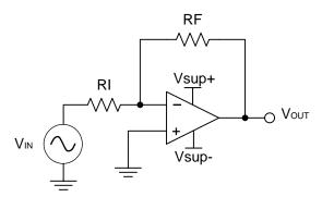
Figure 5. Inverting Amplifier
