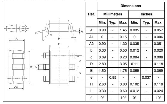
Figure 17. Footprint - dimensions in mm [inches]
