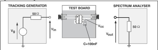
Figure 16 gives the measurement circuit for the analog application. In usual frequency range of analog signals (up to 240 MHz) the effect on disturbed line is less than -45 dB (see Figure 8).
