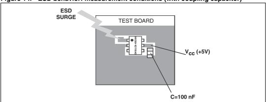
Figure 14. ESD behavior: measurement conditions (with coupling capacitor)
