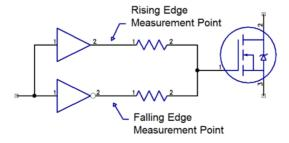
Figure 10: Measurement points for rise and fall time.
