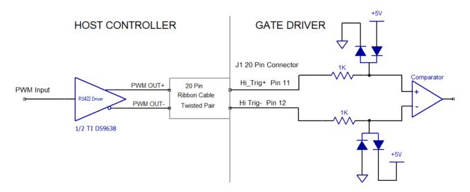
Figure 7: Input buffer schematic - differential input
