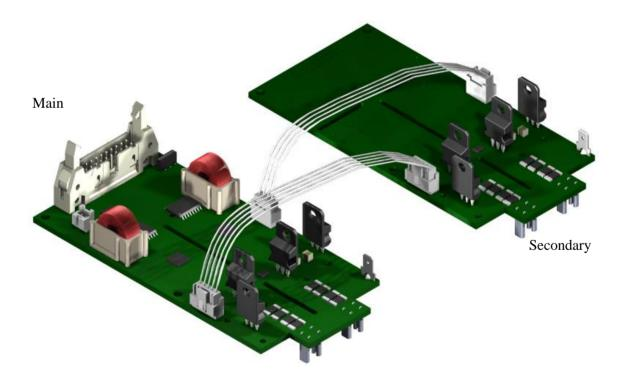
Figure 5: Typical Main-Secondary Setup
