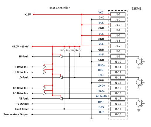
Figure 3: 20 pin pinout diagram for 62EM1-62mm Electrical Gate Driver
