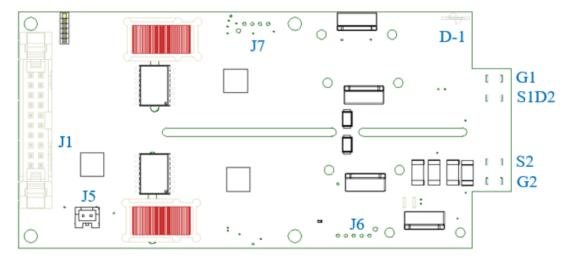
Figure 3: Interconnect Locations on PCB
