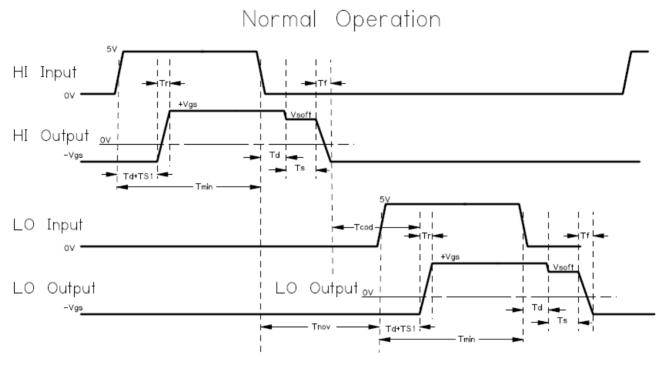
Figure 8: Signal input and output timing diagram.
