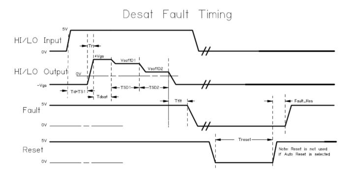
Figure 9: Signal desaturation and fault timing diagram.
