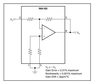
FIGURE 6. Precision Unity-Gain Inverting Amplifier.
