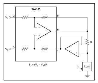
FIGURE 20. Differential Input Voltage-to-Current Converter for Low  $\rm I_{OUT}.$
