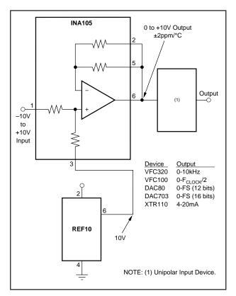
FIGURE 15. Precision Bipolar Offsetting.
