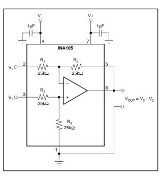
FIGURE 1. Basic Power Supply and Signal Connections.
