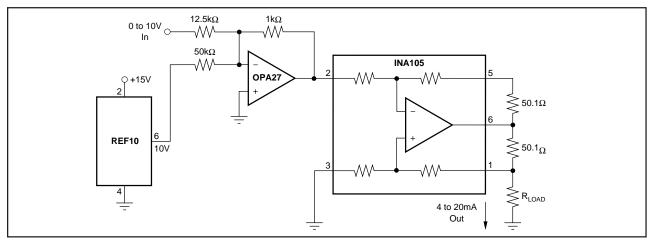
FIGURE 29. Precision 4-20mA Current Transmitter.
