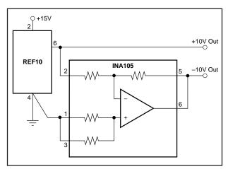
FIGURE 7. ±10V Precision Voltage Reference.
