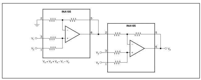
FIGURE 18. Precision Summing Instrumentation Amplifier.
