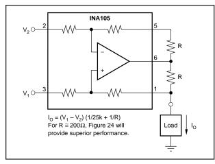
FIGURE 19. Precision Voltage-to-Current Converter with Differential Inputs.
