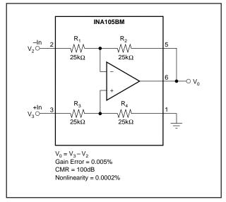
FIGURE 3. Precision Difference Amplifier.
