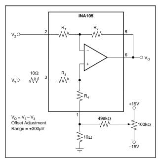
FIGURE 2. Offset Adjustment.
