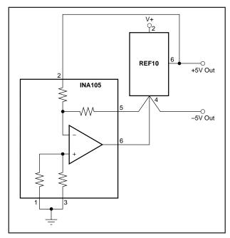
FIGURE 8. ±5V Precision Voltage Reference.
