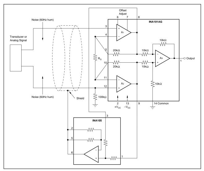
FIGURE 17. Instrumentation Amplifier Guard Drive Generator.
