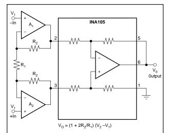
For low source impedance applications, an input stage using OPA27 op amps will give the best low noise, offset, and temperature drift performance. At source impedances above about 10kΩ, the bias current noise of the OPA27 reacting with the input impedance begins to dominate the noise performance. For these applications, using the OPA111 or dual OPA2111 FET input op amp will provide lower noise performance. For lower cost use the OPA121 plastic. To construct an electrometer use the OPA128.
