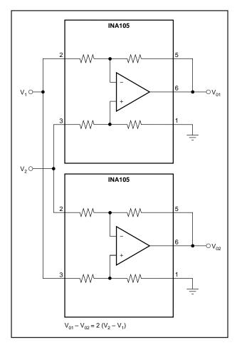
FIGURE 22. Differential Output Difference Amplifier.
