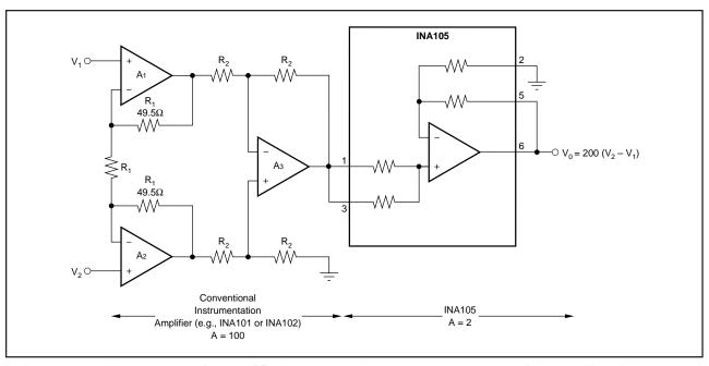
FIGURE 27. Boosting Instrumentation Amplifier Common-Mode Range From ±5 to ±7.5V with 10V Full-Scale Output.
