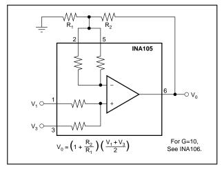
FIGURE 16. Precision Summing Amplifier with Gain.
