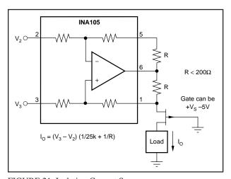
FIGURE 21. Isolating Current Source.
