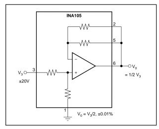
FIGURE 14. Precision Gain = 1/2 Amplifier.
