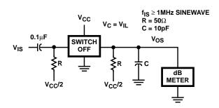
FIGURE 7. SWITCH OFF SIGNAL FEEDTHROUGH TEST CIRCUIT
