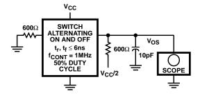
FIGURE 6. CONTROL-TO-SWITCH FEEDTHROUGH NOISE TEST CIRCUIT
