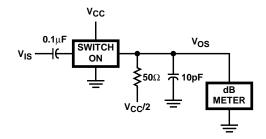
FIGURE 4. FREQUENCY RESPONSE TEST CIRCUIT
