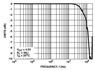
FIGURE 2. TYPICAL SWITCH FREQUENCY RESPONSE
