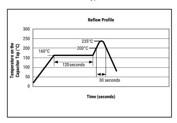
Above "Reflow Profile" graph indicates temperature at capacitor top.
