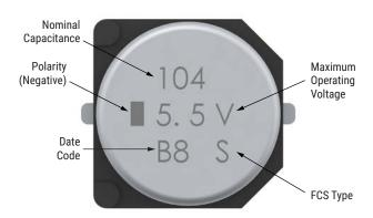
Displays nominal capacitance, maximum operating voltage serial number, polarity, etc.
