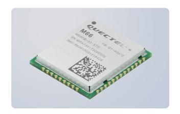
M66 R2.0 is an ultra-compact quad-band GSM/GRPS module using LCC castellation packaging. Based on the latest 2G chipset, it has the optimal performance in SMS & data transmission and audio service even in harsh environment. The highly compact 17.7mm × 15.8mm × 2.3mm profile makes it a perfect platform for size sensitive applications.
