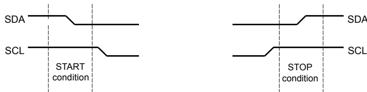
Figure 21-3. START and STOP Conditions
