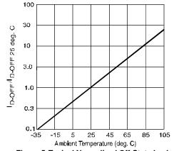
Figure 5. Typical Normalized Off-State Leakage
