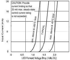
Figure 6. Input Characteristics (Current Controlled)
