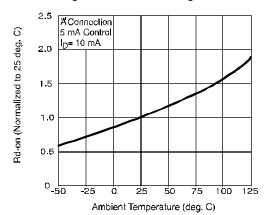
Figure 4. Typical Normalized On-Resistance
