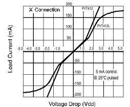
Figure 3. Linearity Characteristics
