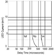
Figure 7. Typical Delay Times
