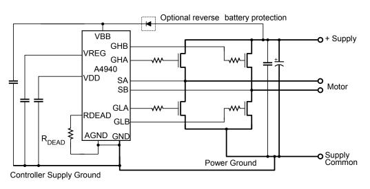
Figure 2. Supply routing suggestions
