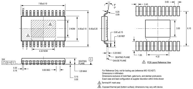
Reference land pattern layout (reference IPC7351 TSOP65P640X120-25M); all pads a minimum of 0.20 mm from all adjacent pads; adjust as necessary to meet application process requirements and PCB layout tolerances; when mounting on a multilayer PCB, thermal vias at the exposed thermal pad land can improve thermal dissipation (reference EIA/JEDEC Standard JESD51-5)
