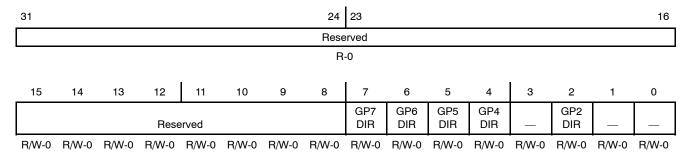
$\textbf{Legend:} \quad \text{R/W} = \text{Readable/Writeable; } -n = \text{value after reset, } -x = \text{undefined value after reset}$
