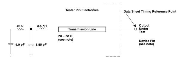
NOTE: The data sheet provides timing at the device pin. For output timing analysis, the tester pin electronics and its transmission line effects must be taken into account. A transmission line with a delay of 2 ns or longer can be used to produce the desired transmission line effect.
