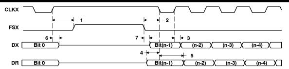
Figure 46. McBSP Timing as SPI Master or Slave: CLKSTP = 11b, CLKXP = 1
