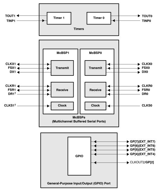
$<sup>^{\</sup>dagger}$  For proper device operation, these pins must be externally pulled up with a 10-k $\!\Omega$  resistor.
