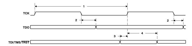
Figure 49. JTAG Test-Port Timing
