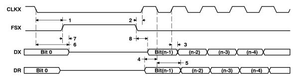
Figure 43. McBSP Timing as SPI Master or Slave: CLKSTP = 10b, CLKXP = 0
