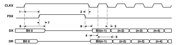
Figure 45. McBSP Timing as SPI Master or Slave: CLKSTP = 10b, CLKXP = 1
