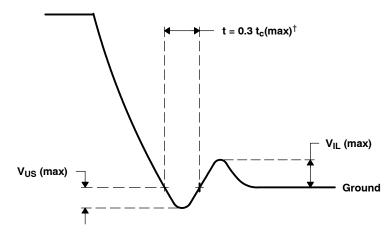
Figure 19. AC Transient Specification Fall Time
