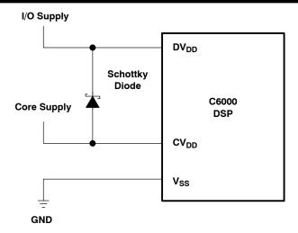
Figure 13. Schottky Diode Diagram
