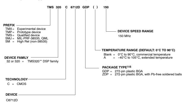
Figure 5. TMS320C6000™ DSP Platform Device Nomenclature (Including the TMS320C6712D Device)
