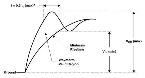
Figure 18. AC Transient Specification Rise Time
