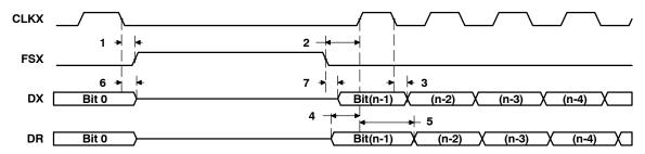
Figure 44. McBSP Timing as SPI Master or Slave: CLKSTP = 11b, CLKXP = 0
