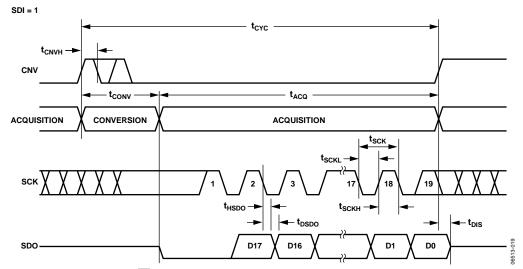
Figure 32. CS Mode, 3-Wire with Busy Indicator Serial Interface Timing (SDI High)
