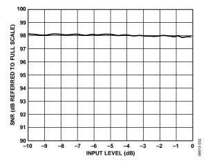
Figure 11. SNR vs. Input Level
