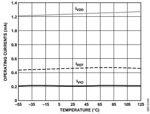
Figure 20. Operating Currents vs. Temperature
