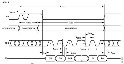
Figure 30. CS Mode, 3-Wire Without Busy Indicator Serial Interface Timing (SDI High)
