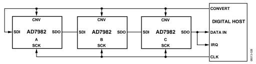
Figure 39. Chain Mode with Busy Indicator Connection Diagram
