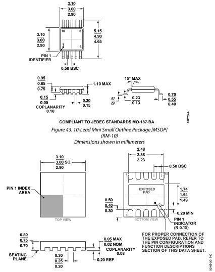
Figure 44. 10-Lead Lead Frame Chip Scale Package [QFN (LFCSP\_WD)] 3 mm × 3 mm Body, Very Very Thin, Dual Lead (CP-10-9)
