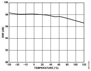
Figure 13. SNR vs. Temperature
