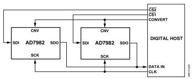
Figure 33. CS Mode, 4-Wire Without Busy Indicator Connection Diagram
