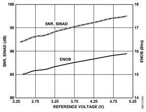
Figure 12. SNR, SINAD, and ENOB vs. Reference Voltage
