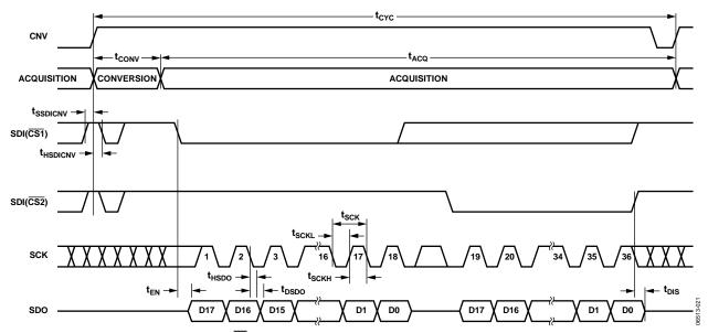
Figure 34. CS Mode, 4-Wire Without Busy Indicator Serial Interface Timing
