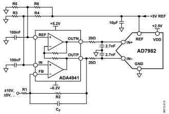
Figure 26. Single-Ended-to-Differential Driver Circuit
