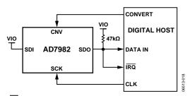
Figure 31. CS Mode, 3-Wire with Busy Indicator Connection Diagram (SDI High)
