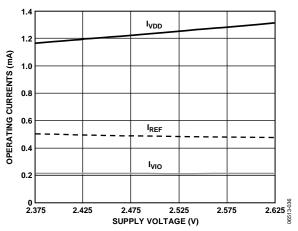
Figure 18. Operating Currents vs. Supply Voltage
