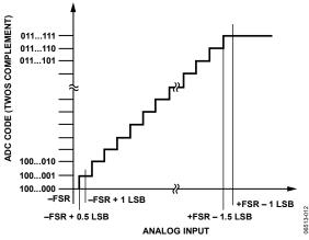
Figure 22. ADC Ideal Transfer Function
