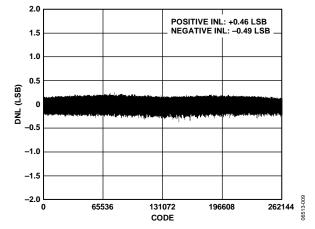
Figure 9. Differential Nonlinearity vs. Code
