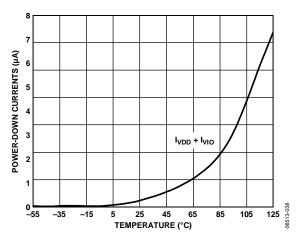
Figure 19. Power-Down Currents vs. Temperature
