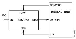
Figure 29. CS Mode, 3-Wire Without Busy Indicator Connection Diagram (SDI High)
