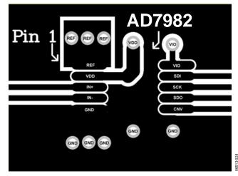
Figure 41. Example Layout of the AD7982 (Top Layer)
