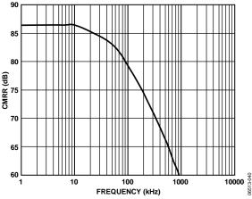
Figure 25. Analog Input CMRR vs. Frequency
