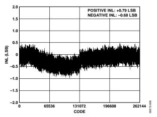
Figure 6. Integral Nonlinearity vs. Code
