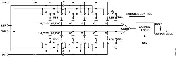
Figure 21. ADC Simplified Schematic
