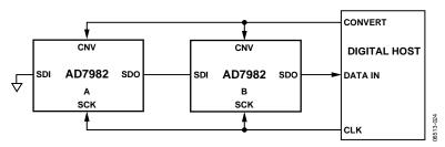
Figure 37. Chain Mode Without Busy Indicator Connection Diagram
