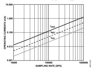
Figure 28. Operating Currents vs. Sampling Rate
