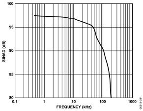
Figure 14. SINAD vs. Frequency
