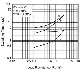
SWITCHING TIME vs. LOAD RESISTANCE
