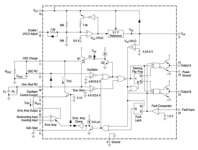
Figure 14. MC34067 Representative Block Diagram
