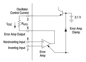
Figure 17. Error Amplifier and Clamp
