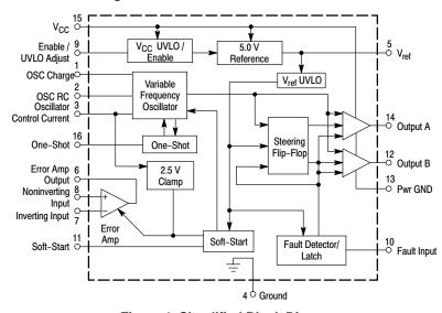
Figure 1. Simplified Block Diagram
