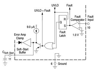
Figure 20. Fault Detector and Soft-Start
