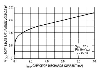
Figure 11. Soft-Start Saturation Voltage versus Capacitor Discharge Current
