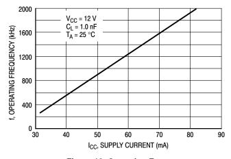
Figure 12. Operating Frequency versus Supply Current
