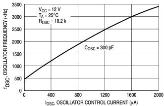
Figure 3. Oscillator Frequency versus
