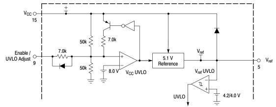
Figure 19. Undervoltage Lockout and Reference
