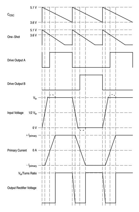
Figure 21. Application Timing Diagram
