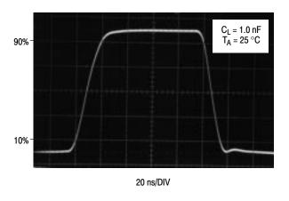
Figure 10. Drive Output Waveform
