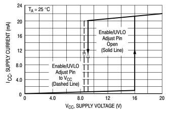
Figure 13. Supply Current versus Supply Voltage
