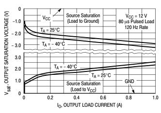
Figure 9. Drive Output Saturation Voltage versus Load Current
