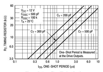
Figure 5. One-Shot Timing Resistor versus Period
