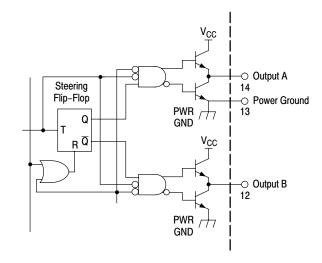
Figure 18. Steering Flip-Flop and Output Drivers
