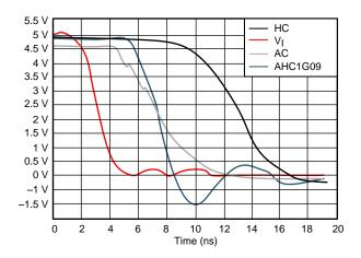
$V_{CC} = 5 \text{ V}, \text{ Load} = 50 \Omega / 50 \text{ pF}$
