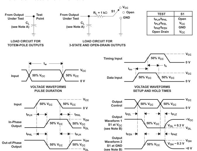
A. C<sub>L</sub> includes probe and jig capacitance.
