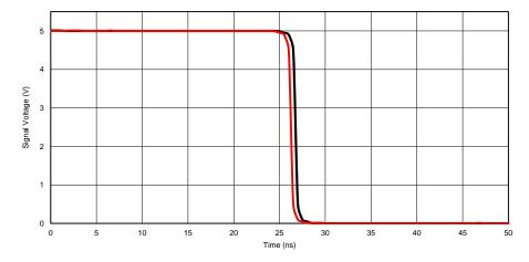
Figure 1. TPD Across V<sub>CC</sub> at 25°C
