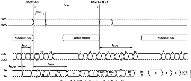
Figure 42. Self Clocked Interface Mode Timing Diagram
