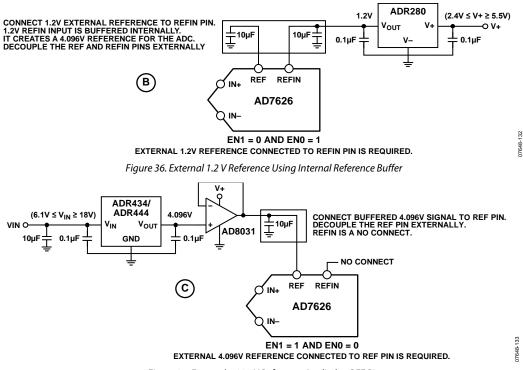
Figure 37. External 4.096 V Reference Applied to REF Pin
