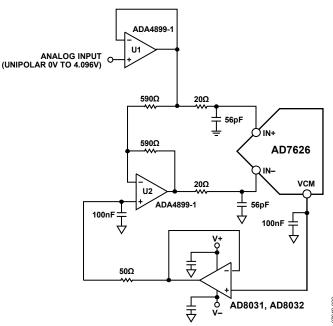
Figure 32. Single-Ended to Differential Driver Circuit Using ADA4899-1
