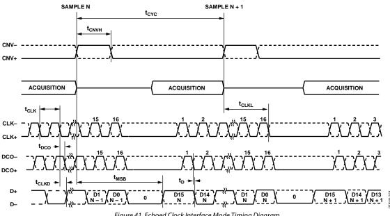
Figure 41. Echoed Clock Interface Mode Timing Diagram
