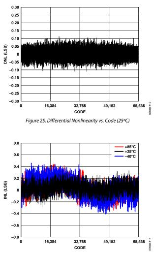
Figure 26. Integral Nonlinearity vs. Code vs. Temperature
