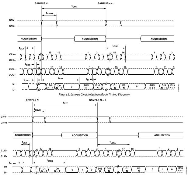
Figure 3. Self Clocked Interface Mode Timing Diagram
