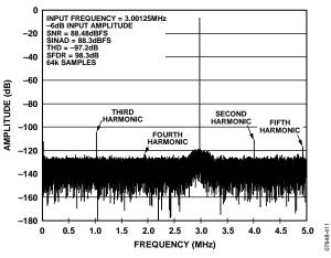
Figure 10. FFT, 3 MHz, –6 dB Input Tone, Wide View
