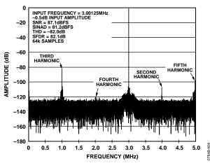
Figure 7. FFT, 3 MHz, –0.5 dB Input Tone, Wide View
