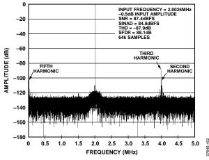
Figure 6. FFT, 2 MHz, -0.5 dB Input Tone, Wide View
