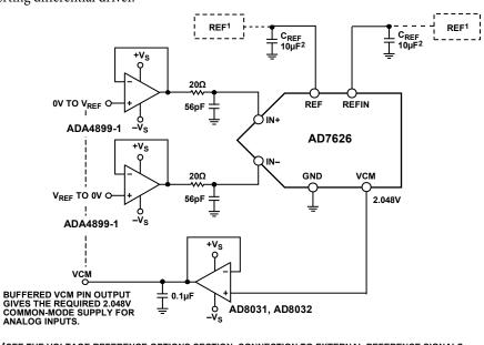
$^1$ SEE THE VOLTAGE REFERENCE OPTIONS SECTION. CONNECTION TO EXTERNAL REFERENCE SIGNALS IS DEPENDENT ON THE EN1 AND EN0 SETTINGS.  $^2C_{REF}$  IS USUALLY A 10µF CERAMIC CAPACITOR WITH LOW ESL AND ESR.
