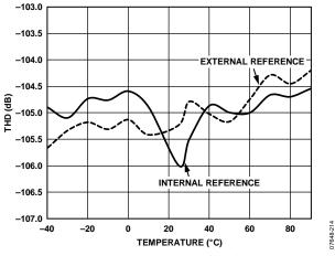
Figure 19. THD vs. Temperature (-0.5 dB, 20 kHz Input Tone)
