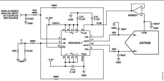
Figure 34. High Frequency Input Drive Circuit Using the ADA4932-1; Single-Ended to Differential Configuration
