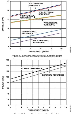
Figure 40. Power Dissipation vs. Sampling Rate
