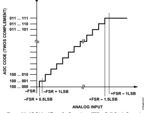
Figure 28. ADC Ideal Transfer Functions (FSR = Full-Scale Range)
