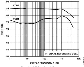
Figure 38. PSRR vs. Supply Frequency (350 mV p-p Ripple on VDD2, 600 mV Ripple on VDD1)
