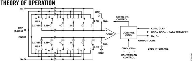
Figure 27. ADC Simplified Schematic
