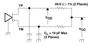
NOTE A: The lumped instrumentation capacitance for any single-ended voltage measurement is less than or equal to 10 pF. When making measurements at YP or YM, the complementary output is similarly loaded.
