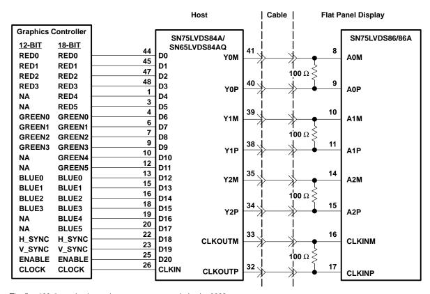
NOTES: A. The five 100- $\Omega$  terminating resistors are recommended to be 0603 types.
