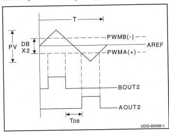
Figure 2. Oscillator and PWM Waveforms
