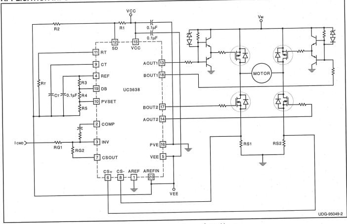
Figure 1. Average Motor Current Control Loop
