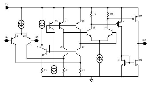
Figure 3. Simplified Schematic
