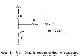
ote 1:  $R \le 10 \text{ k}\Omega$  is recommended. A suggested starting value is  $10 \text{ k}\Omega$ . Ensure that the MCLR pin VIH and VIL specifications are met.
