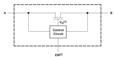
(1) Gate voltage (V<sub>G</sub>) is equal to approximately V<sub>CC</sub> + V<sub>T</sub> when the switch is ON and  $V_I > V_{CC} + V_T$ . (2) EN is the internal enable signal applied to the switch.
