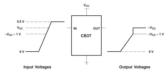
NOTE A: If the input high voltage ( $V_{IH}$ ) level is greater than or equal to  $V_{CC} - 1$  V, and less than or equal to 5.5 V, then the output high voltage ( $V_{OH}$ ) level will be equal to approximately the  $V_{CC}$  voltage level.
