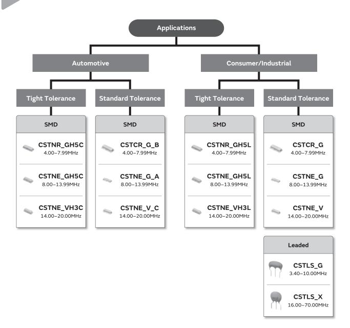
Notice: "CERALOCK for consumer" and "CERALOCK for automotive" is different in the specification of Operating Temperature Range, Environmental Characteristics, Physical Characteristics and so on. Please choose either "for consumer" or "for automotive" according to the required specification.
