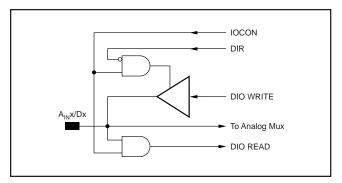
FIGURE 7. Analog/Data Interface Pin.
