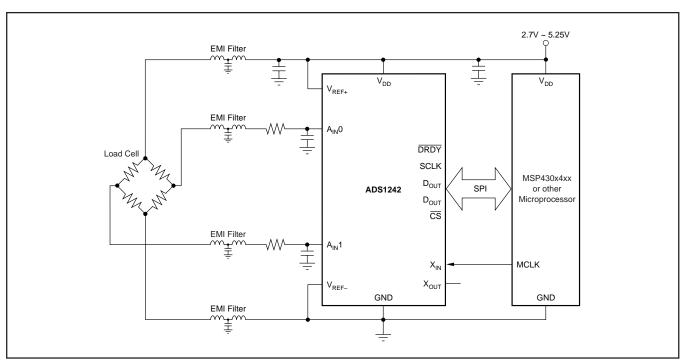
FIGURE 8. Schematic of a General-Purpose Weight Scale.
