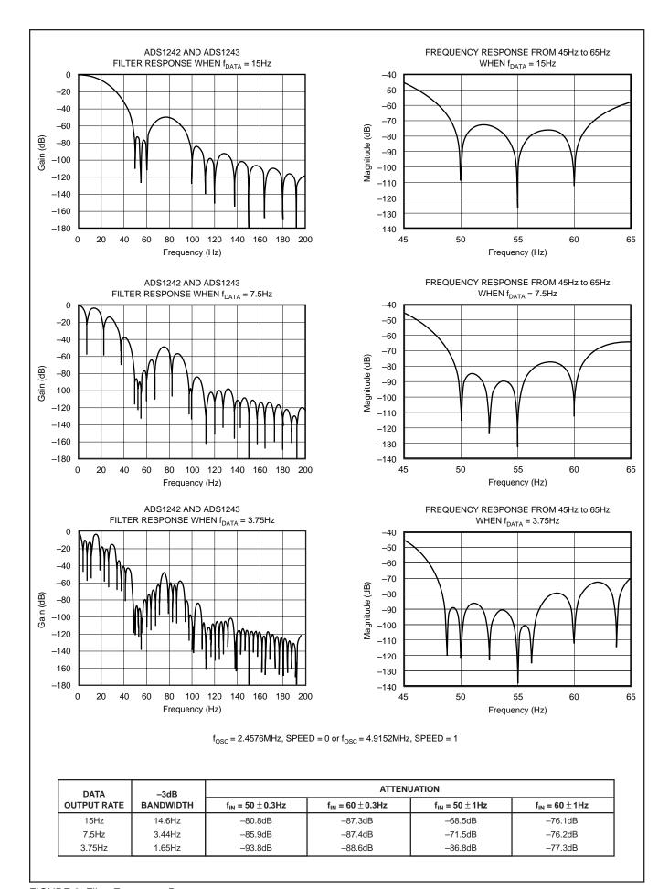
FIGURE 6. Filter Frequency Responses.
