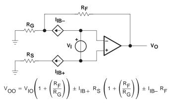
Figure 37. Output Offset Voltage Model
