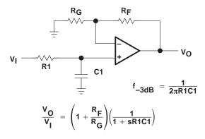
Figure 38. Single-Pole Low-Pass Filter
