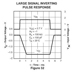
LARGE SIGNAL INVERTING PULSE RESPONSE
