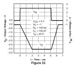
SMALL SIGNAL INVERTING PULSE RESPONSE
