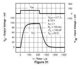
LARGE SIGNAL INVERTING PULSE RESPONSE
