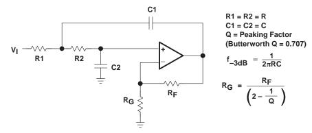
Figure 39. 2-Pole Low-Pass Sallen-Key Filter
