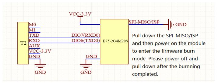
Notes: The diagram shows that the module needs to be connected to the USB to UART module to download the firmware.
