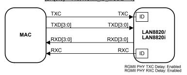
Strapping RGMII\_ID\_MODE high sets the device into Hybrid Mode. In order to set the device into ID Mode, the RGMII PHY TXC Delay Enable and RGMII PHY RXC Delay Enable bits of the Control / Status Indications Register (27.[9:8]) must be configured via software to 01b.
