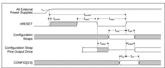
FIGURE 5-3: HARDWARE RESET TIMING
