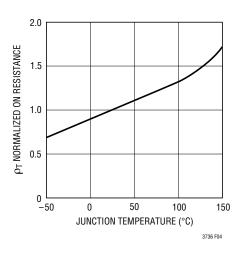
Figure 4. R<sub>DS(ON)</sub> vs Temperature
