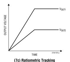
Figures 7b and 7c. Two Different Modes of Output Voltage Tracking
