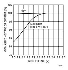
Figure 12. Line Regulation of V<sub>REF</sub> and Maximum Sense Voltage for Low Input Supply
