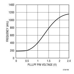
Figure 8. Relationship Between Oscillator Frequency and Voltage at the PLLLPF Pin When Synchronizing to an External Clock
