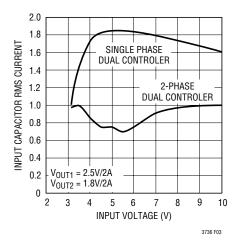
Figure 3. RMS Input Current Comparison
