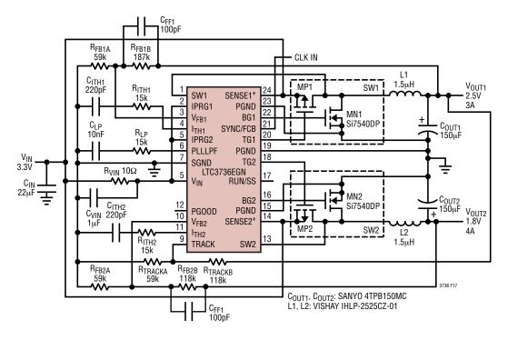
Figure 17. 2-Phase, Synchronizable, Dual Output Synchronous DC/DC Converter
