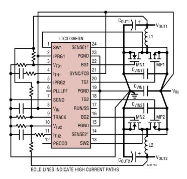
Figure 13. LTC3736 Layout Diagram
