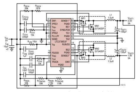
Figure 15. 2-Phase, 550kHz, Dual Output Synchronous DC/DC Converter
