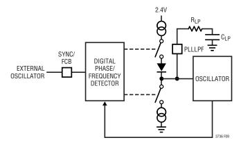
Figure 9. Phase-Locked Loop Block Diagram
