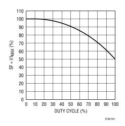
Figure 1. Maximum Peak Current vs Duty Cycle
