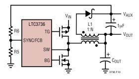
Figure 10. Auxiliary Output Loop Connection
