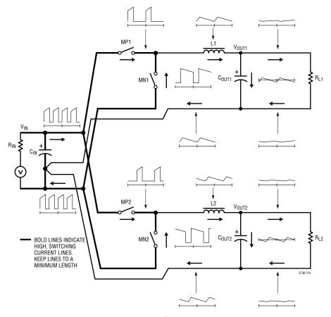
Figure 14. Branch Current Waveforms
