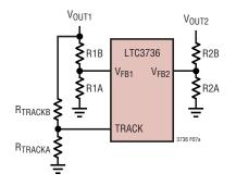
Figure 7a. Using the TRACK Pin
