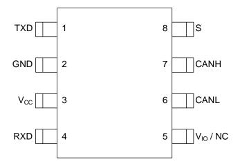
Figure 6-1 CA-IF1051S/VS Pin Configuration
