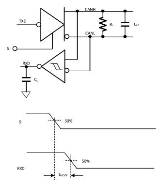
Figure 8-4 Mode Change Test Circuit and Timing Diagram
