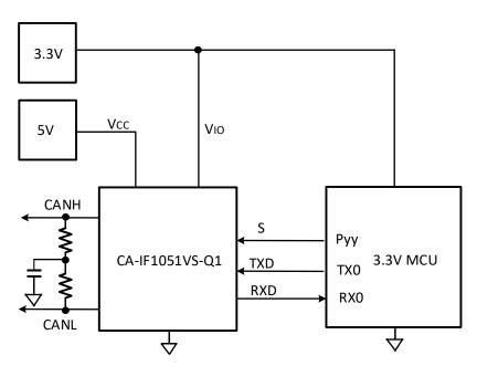
Figure 10- 1 CA-IF1051VS-Q1 Typical Application Circuit
