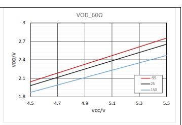
Figure 7-7 Differential Output Voltage vs.  $V_{CC}$  ( $R_L = 60\Omega$ )
