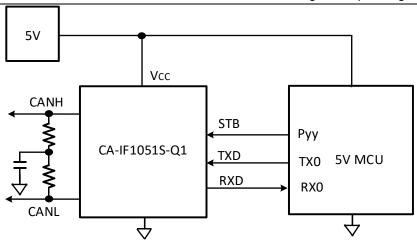
Figure 10-2 CA-IF1051S-Q1 Typical Application Circuit
