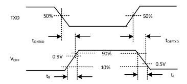
Figure 8-1 Transmitter Test Circuit and Timing Diagram
