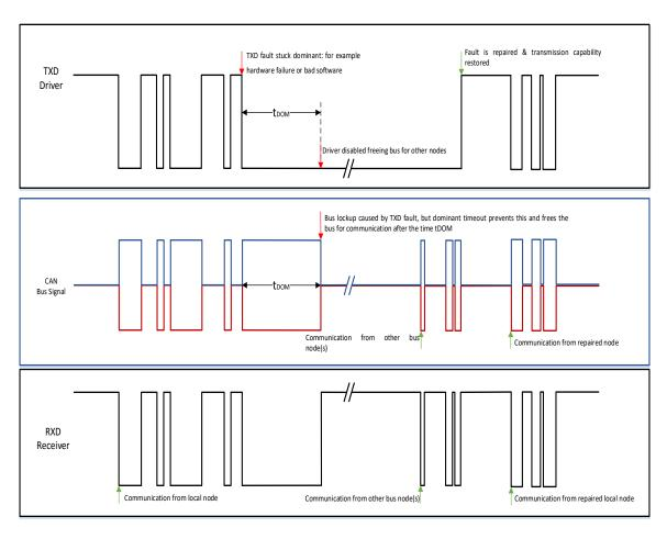
Figure 9-2 Transmitter-Dominant Timeout Protection
