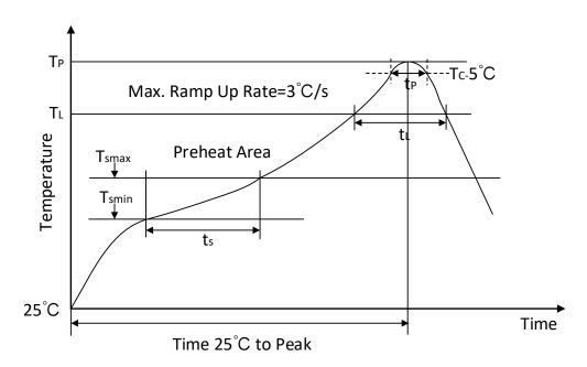
Figure 12- 3 Soldering Temperature (reflow) Profile
