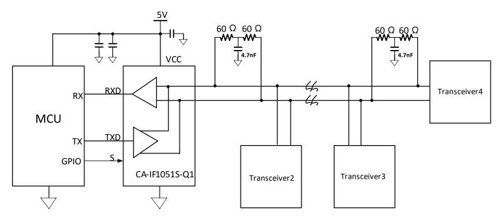
Figure 10-3 Typical CAN bus Network
