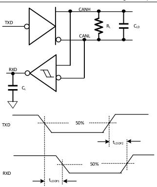
Figure 8-3 TXD to RXD Loop Delay
