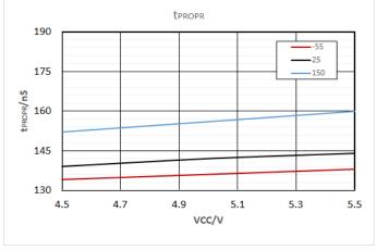
Figure 7-9 Loop Delay, Recessive to Dominant
