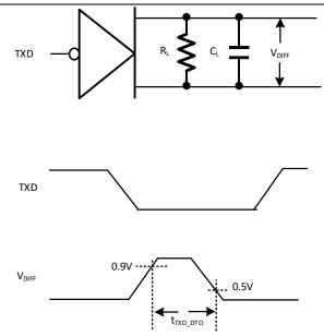
Figure 8-5 Transmitting Dominant Timeout Timing Diagram
