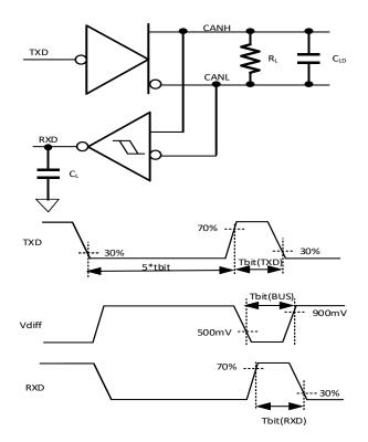
Figure 8-6 CAN FD Timing Parameter Measurement
