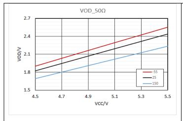
Figure 7-6 Differential Output Voltage vs.  $V_{CC}$  (R<sub>L</sub> = 50 $\Omega$ )
