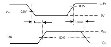
Figure 8-2 Receiver Test Circuit and Timing Diagram
