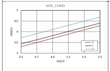
Figure 7-8 Differential Output Voltage vs.  $V_{CC}$  ( $R_L = 240\Omega$ )
