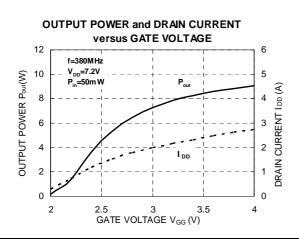
**OUTPUT POWER and DRAIN CURRENT** versus GATE VOLTAGE f=350MHz V<sub>DD</sub>=7.2V OUTPUT POWER Pout (W) P. = 50m W I DD (A) DRAIN CURRENT
