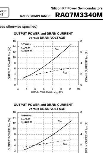
**TYPICAL PERFORMANCE** ( $T_{case}$ =+25°C,  $Z_G$ = $Z_L$ =50 $\Omega$ , unless otherwise specified)
