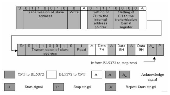
II) The second method to reading data from the internal register is to start immediately after writing to the internal address pointer and the transmission format register. Set 4h to the transmission format register when this method is used.
