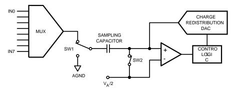
Figure 34. ADC128S022 in Track Mode
