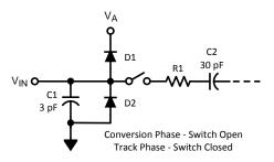
Figure 37. Equivalent Input Circuit
