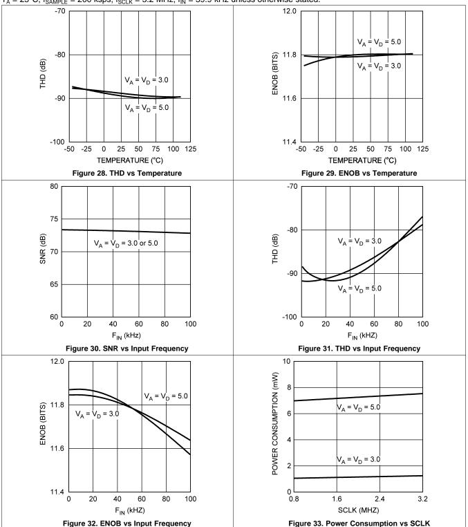
$T_A = 25^{\circ}C$ ,  $f_{SAMPLE} = 200$  ksps,  $f_{SCLK} = 3.2$  MHz,  $f_{IN} = 39.9$  kHz unless otherwise stated.
