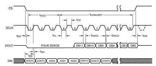
Figure 2. ADC128S022 Serial Timing Diagram
