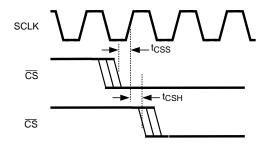
Figure 3. SCLK and  $\overline{CS}$  Timing Parameters
