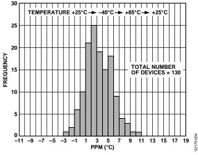
Figure 4. ADR380 Output Voltage Temperature Coefficient
