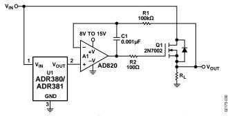
Figure 30. ADR380/ADR381 for Precision High Current Voltage Source
