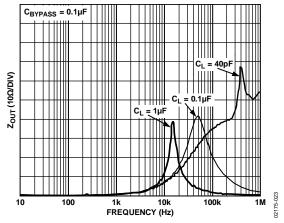
Figure 23. ADR381 Output Impedance vs. Frequency
