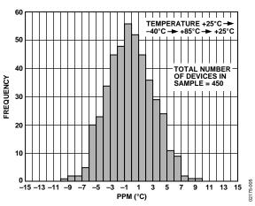
Figure 5. ADR381 Output Voltage Temperature Coefficient
