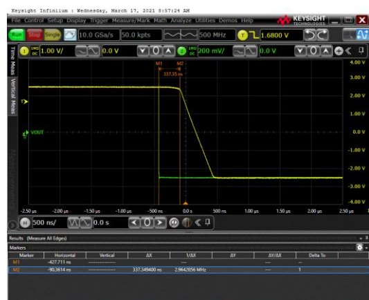
Figure 16 Overload Recovery at Positive Rail
