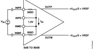
Figure 41. Input Voltage Applied to the INPR and INMR Pins
