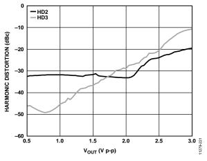
Figure 21. Harmonic Distortion vs. Output Amplitude
