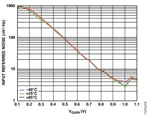
Figure 18. Input Referred Noise vs. VGAIN
