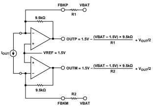
Figure 47. Decreasing the Output Common-Mode Voltage
