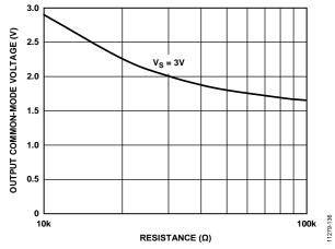
Figure 38. Output Common-Mode Voltage vs.  $R_{CM}$  to COMM
