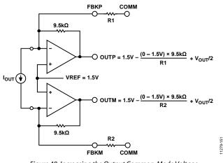
Figure 48. Increasing the Output Common-Mode Voltage
