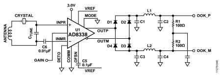
Figure 49. Complete, Low Power OOK Receiver
