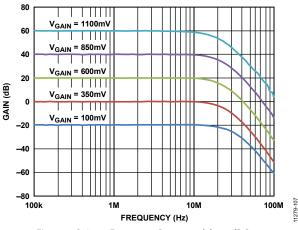
Figure 8. Gain vs. Frequency,  $R_{IN} = 2 \times 5 \ k\Omega$ , 20 dB Steps
