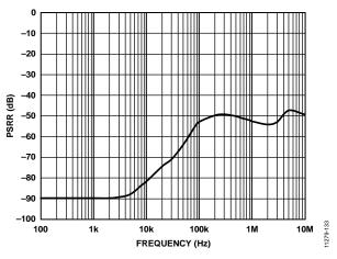
Figure 34. Power Supply Rejection Ratio (PSRR) vs. Frequency
