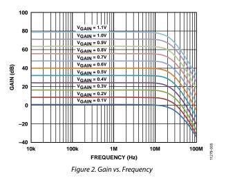
The AD8338 offers additional versatility by providing access to the internal summing nodes of the VGA core and the output amplifiers. With the addition of a few external passive components, users can customize the gain, bandwidth, input impedance, and noise profile of the device to fit their application.
