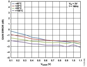
Figure 9. Gain Error vs. V<sub>GAIN</sub> over Temperature
