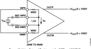
Figure 43. Using External Resistors at the INPD and INMD Pins
