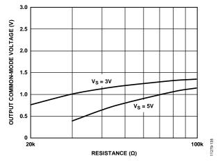
Figure 37. Output Common-Mode Voltage vs. Common-Mode Resistance (R<sub>CM</sub>) to VBAT
