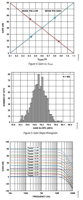
Figure 6. Gain vs. Frequency, 8 dB Steps
