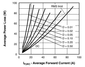
Fig. 6 - Forward Power Loss Characteristics
