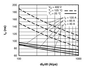
Fig. 7 - Typical Reverse Recovery Time vs. di<sub>F</sub>/dt
